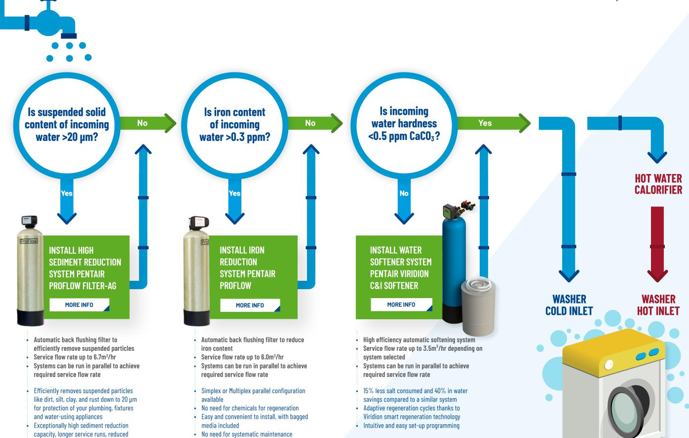
Lower backwash flow rate, reduced backwash water consumption
