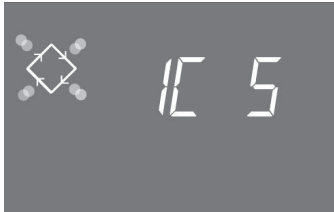
Cycle in progress and time remaining before going on to the next cycle. In this example the cycle in progress is the first one and 5 minutes remains before switching the valves to the second regeneration cycle.
