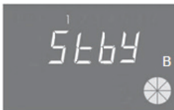
In regeneration status – Stand-by state display
