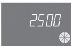
In-service status – volume display
