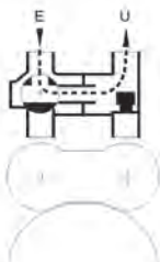
Handmatige bypass - systeem in bypass
