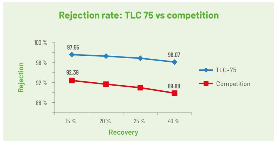
Testing conditions: 75 gallon per day RO membranes, 3.5 bar feed pressure, 1000 ppm of TDS, softened water.
