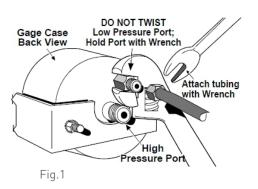
• The "High" pressure port (center mounted) is piped to the Inlet side of the filter. The "Low" pressure port (top center mounted) is piped to the Outlet side of the filter.
