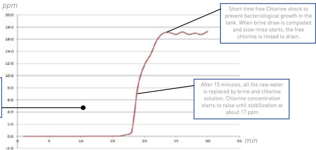
The chlorine production stabilizes after ca.22 minutes with an average value of 17ppm of free CL<sub>2</sub>.
